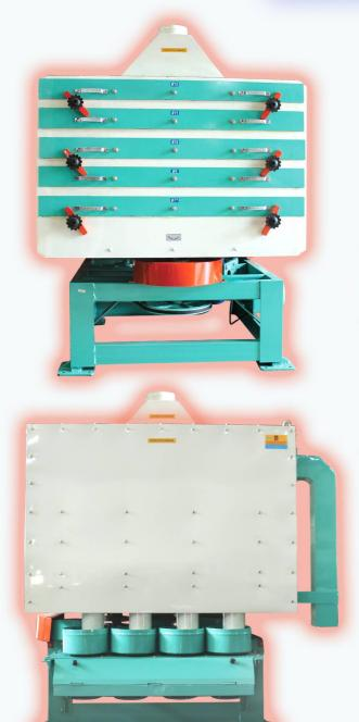
Rice sifter is designed to separate broken rice from head rice. It is equipped with automatic cleaning system and screen can be easily taken out for cleaning in case of heavy clogging.
