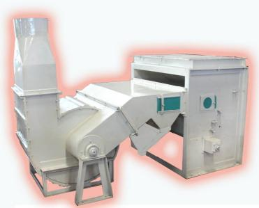
This machine is equipped with dynamically balanced blower which helps in separation of husk. Paddy flows through the adjustable flops to deliver husk free rice and paddy and husk conveyed through the pipe line to husk yard.
