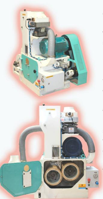
Pneumatic Rubber Sheller is designed to remove husk from all kinds of paddy. This machine comes with heavy- sturdy construction and suitable for raw, steam and boiled paddy. This machine makes very low noise while shelling of paddy
