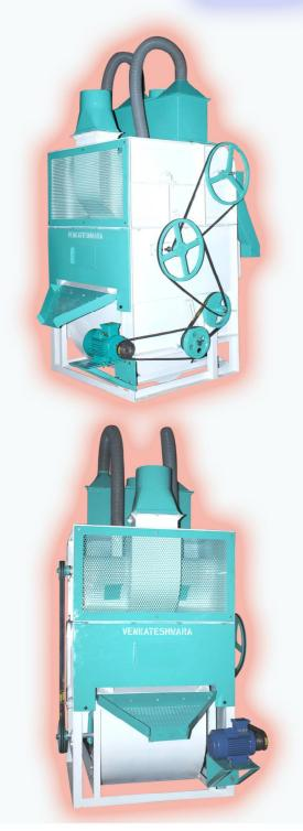
Paddy Cleaner is designed to remove impurities like grains, sticks, straws, big mud lumps and other foreign particles. Paddy Cleaner works more efficiently when paddy is pre cleaned in pre cleaner.
