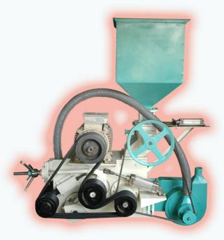
To Increase the rubber rolls life a special cooling blower is attached to the machine.
