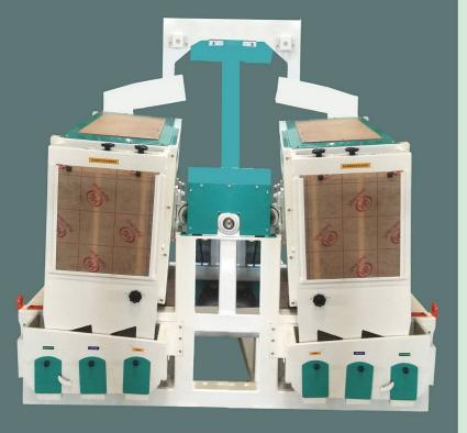
Paddy separator is mainly designed based on gravity to separate paddy and brown rice from the mixture of paddy and brown rice.
