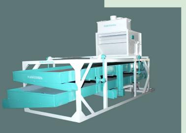
Pre Cleaner is the first cleaner in the rice mill designed to remove all impurities, unfilled grains, seeds and foreign particles from the paddy.
