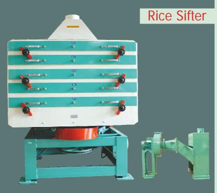
Rice sifter is designed to separate broken rice from head rice. It is equipped with automatic cleaning system and screen can be easily taken out for cleaning in case of heavy clogging.
