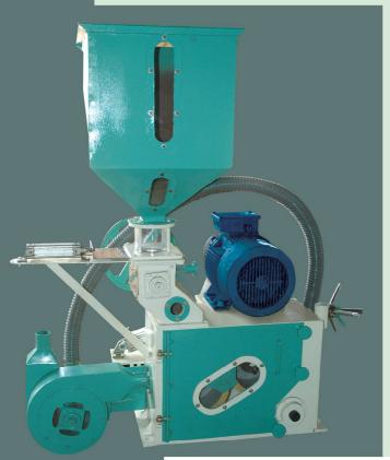
Pneumatic Type Sheller is specially designed to de-husking the paddy. This is fitted with sleeve type rubber drums to maintain better output.
