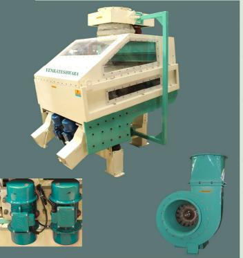
Vibro Paddy Cleaner is designed to remove all impurities, unfilled grains, seeds, stones and foreign particles from the paddy. This machine separates stones and heavy material by density difference.
